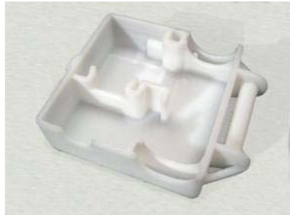
Figure 2: Battery box bottom from Dimension SST.
